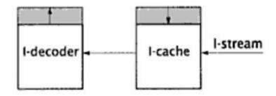
Figure 2.38 I-stream tradeoff: increasing the instruction encoding increases the I-decoder size (area), but decreases the I-cache size (area).
