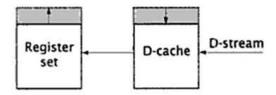
Figure 2.39 D-stream tradeoff: similarly, increasing the register set size decreases the D-cache size.
